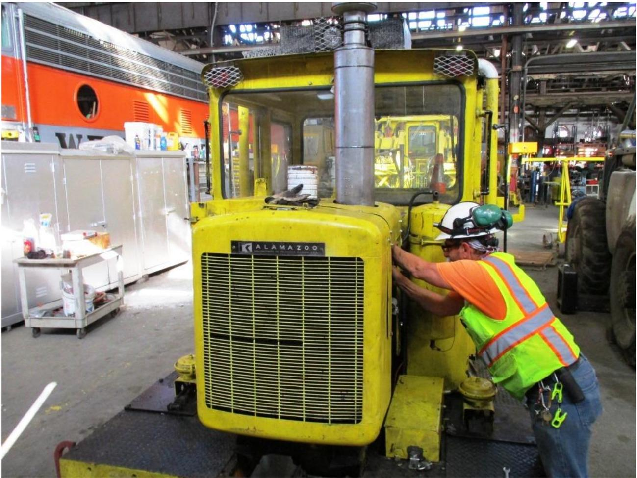
Joe reattaches the muffler to the new engine of the Kalamazoo
